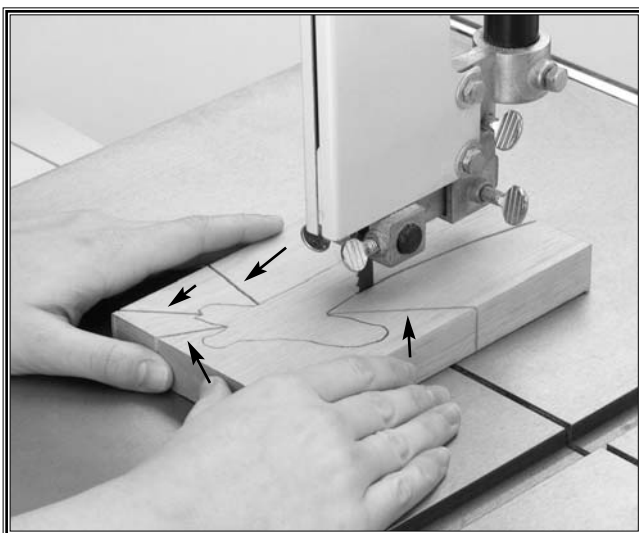
Figure 52. Relief cuts before cutting curves.
